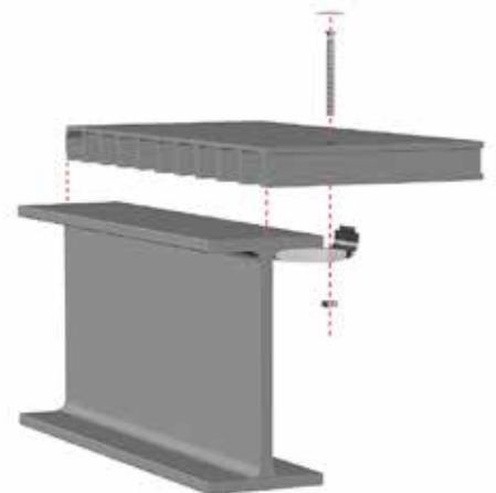
*Typical fixing detail using dome head washer*
