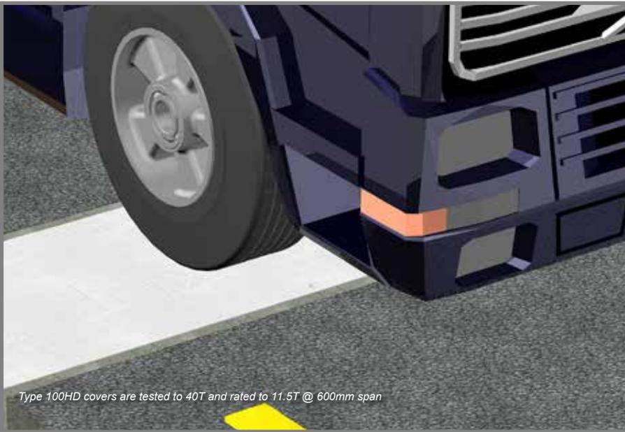
Type 100HD covers are tested to 40T and rated to 11.5T @ 600mm span
